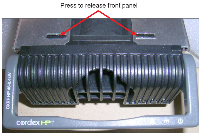
Figure 16 — Removing Front Panel from Rectifier
